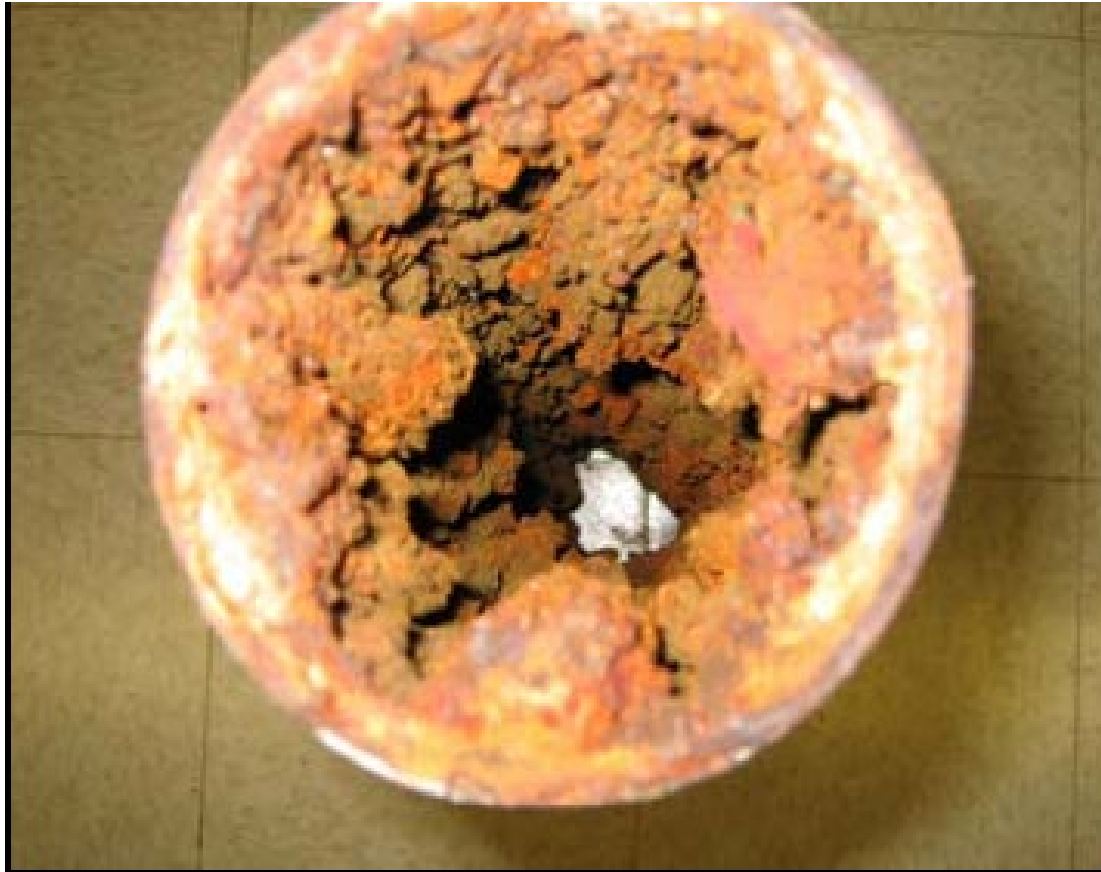
Cross section of 4 inch pipe from hospital hot water system
